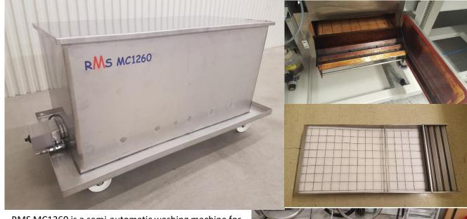
RMS MC1260 is a semi-automatic washing machine for cleaning machine parts, condensation traps, filters, filter holders, soldering frames, soldering pallets etc.
